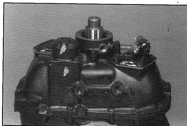
24. Assemble the two spacers and air regulator on the countershaft bearing cap assembly. The air regulator bolts are longer than the bearing cap bolts. Torque the bolts to 34 - 41 ft. lbs.
